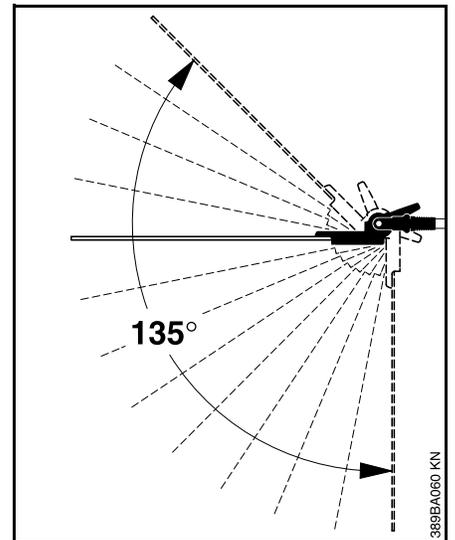
The angle of the cutter bar can be adjusted upwards in 4 stages from 0° (straight) to 45°, and downwards in 8 stages from 0° to 90° (right angle facing down). There are therefore 13 possible working positions.
