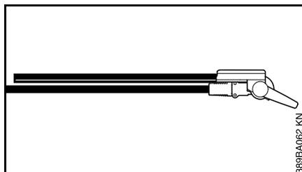
The cutter bar can be folded flat against the drive tube and locked in position to save space during transportation.
