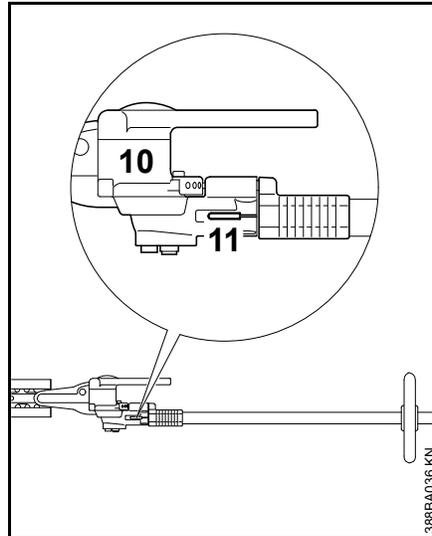
Once the end of the drive tube is inserted beyond the slot in the clamp (11):
