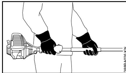
Right hand on control handle, left hand on handle hose on drive tube, even if you are left-handed. Wrap fingers and thumbs firmly around the handles.
