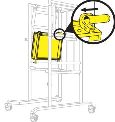
Rotate the platform down and locate the platform claws on the horizontal member of the right hand side frame. Push the platform back towards the back of the unit until it is in contact with the rear folding guardrail frame. Ensure the claws are sitting on the tube and not the plates.
