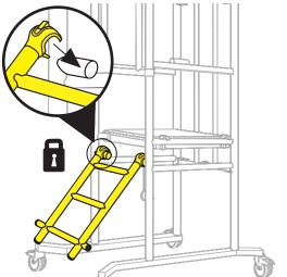
Rotate the ladder down, using the claws as pivots. Locate the bottom of the ladder over the base frame as shown below.
