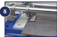
Once scored, position the breaker bar to sit on top of the tile. Ensure the wheel is not in contact with the tile
