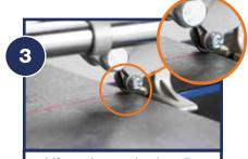
Lift up the scoring handle, check the cutting wheel is on the edge of the tile
