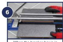
When the breaker bar is in place, apply pressure to the handle – excess force is not needed
