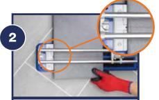
Place the tile on to cutter bed, line up the mark with the centre point indicator
